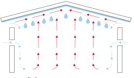
Incorrect ventilation Moist air is not evacuated.
