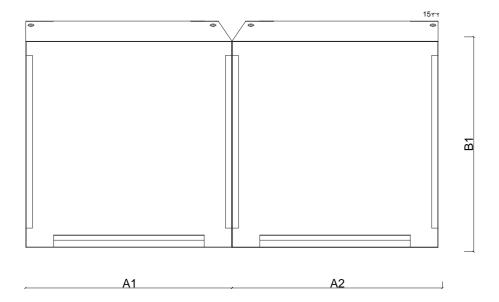
**U-shaped corner panel for vertical installation.**Almax + A2max + A3max = 1000 mm, Almin = 300 mm, A2min = 300 mm, A3min = 300 mm, B1min = 300 mm, B1max = 3000 mm
