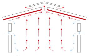
Proper ventilation The vent provides an outlet for moist air.
