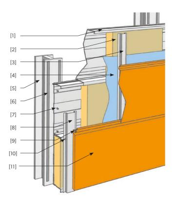
An advantage of curtain walls built using SKRIN cladding cassettes is the fast and uncomplicated assembly. They can be used on any wall as they are hung on a substructure consisting of a steel grate made of P03 20/90 basic profiles.
