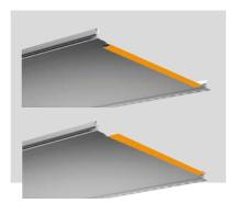
A special panel fold at the eaves part of the roof covers and secures the cut edge and eliminates the need to install screws.
