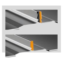
A solution which additionally increases the functionality of the covering is the COVER CAP element, i.e. panel seam caps on both sides. This solution also increases the visual effect and aesthetics of the covering. The COVER CAPs are bent after the installation of the roofing, hiding the visible joint between the sheets and ensuring that the roof presents a uniform, harmonious surface even from up close.
