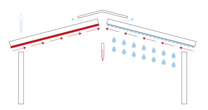
"In the case of buildings, condensation can be enhanced by temperature differences the inside of the building stays warm while the outside temperature drops quickly. The thermally conductive properties of steel roofing cause strong condensation from the warm room on the inside of the roof.
